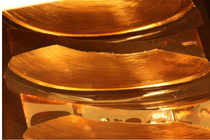
Figure 24. First signs of scuffing on the bronze worm wheel
